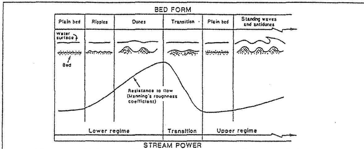
Figure 3.3. Relative resistance in sand-bed channels (after Arcement & Schneider, 1984).
